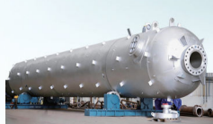
Wastewater Treatment Oxidation Reactor 2023 Jiangsu, China
