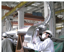
Three-blade Swept-back Type (PVC)
