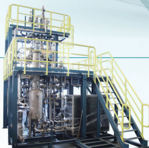
Drying Skid-mounted Equipment
